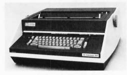
Anderson Jacobson Inc, San Jose manufacturer of data communications equipment, recently announced the availability of its AJ 841. Designed for the dual purpose user, the AJ 841 doubles as both a heavy duty IBM Selectric typewriter and an interactive remote computer terminal.
